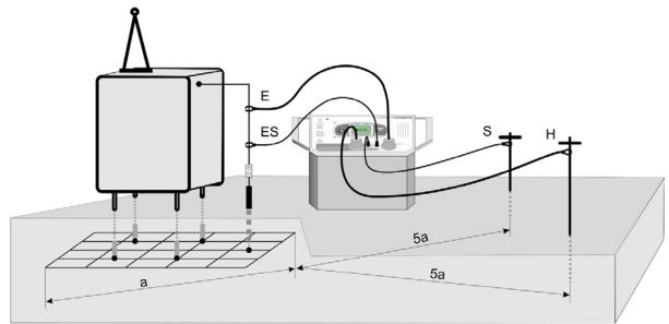
Figure 7.4: Earth resistance measurement
