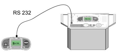
Figure 7.8: Connection of the instruments during synchronization
