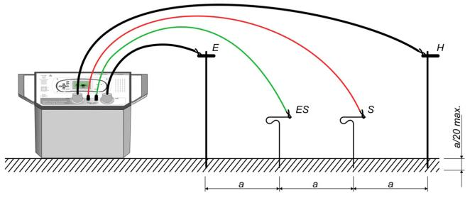
Figure 7.5: Specific earth resistance measurement
