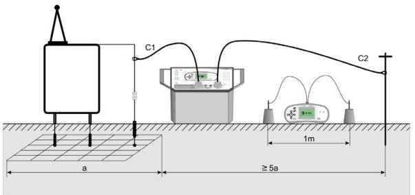
Figure 7.2: Step voltage measurement
