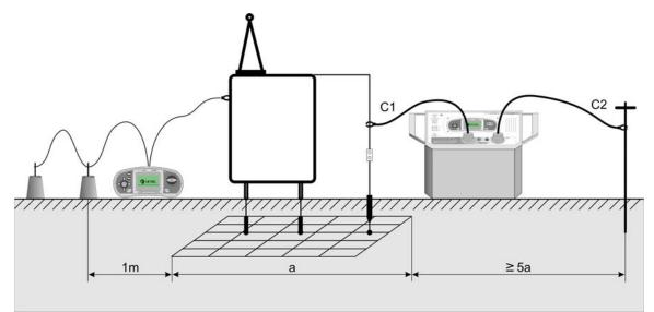
Figure 7.3: Contact voltage measurement
