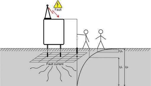
Figure 7.1: Dangerous voltages on a faulty earthing system
